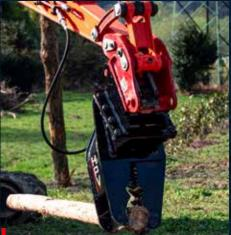
The grab lifts the pile and with a light pressure places it on the ground.
